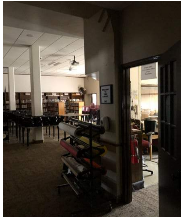
Library only has one exit. A space of this size requires a second exit.
